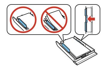
**Note:** Make sure the paper is under the tabs on the edge guides.
